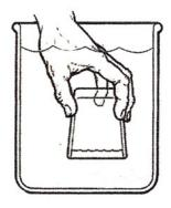
By totaling sealing the Body of the Tail Light and leaving the area open at the bottom, our products use the "Air Trapping" Design using the simple Physics "P-V-T" relationship, which shows by compressing air when Light is submerged, water is only allowed to go up the Light skirt less than 1/4" – regardless of waves – or no waves – TRY\* this principle by tucking tissue into a "glass" and submerging it into 1 to 2 feet of water.
